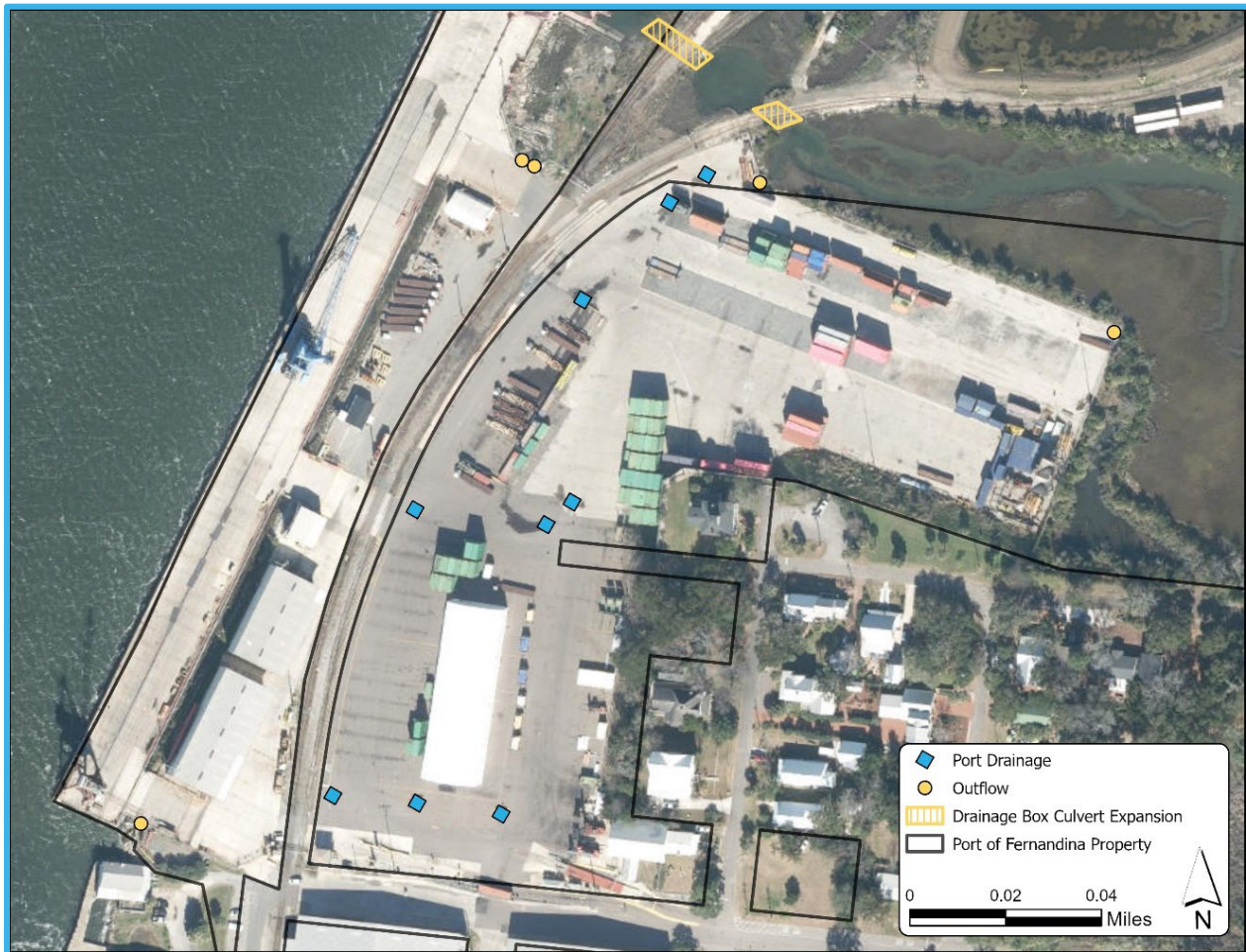
Figure 29 - Improved Drainage and Water Management System
