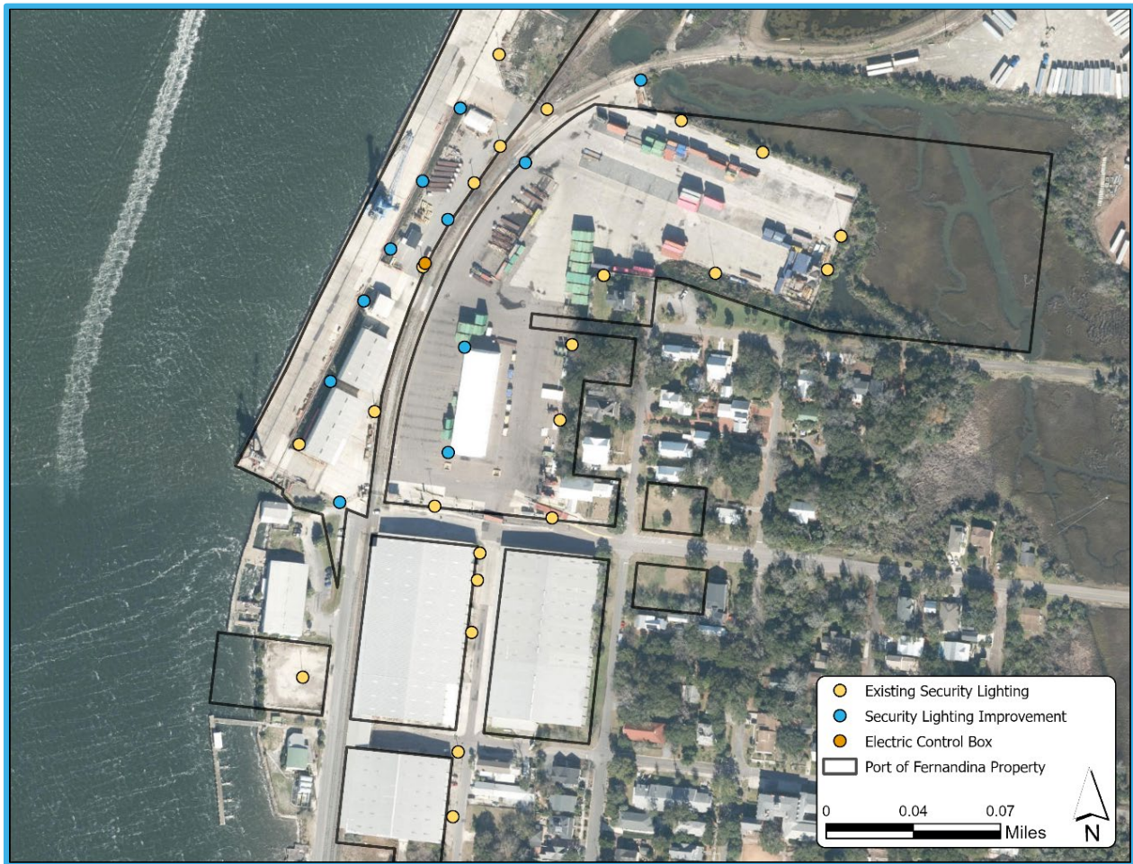
Figure 28 - Port Enhanced Lighting for Security and Safety
