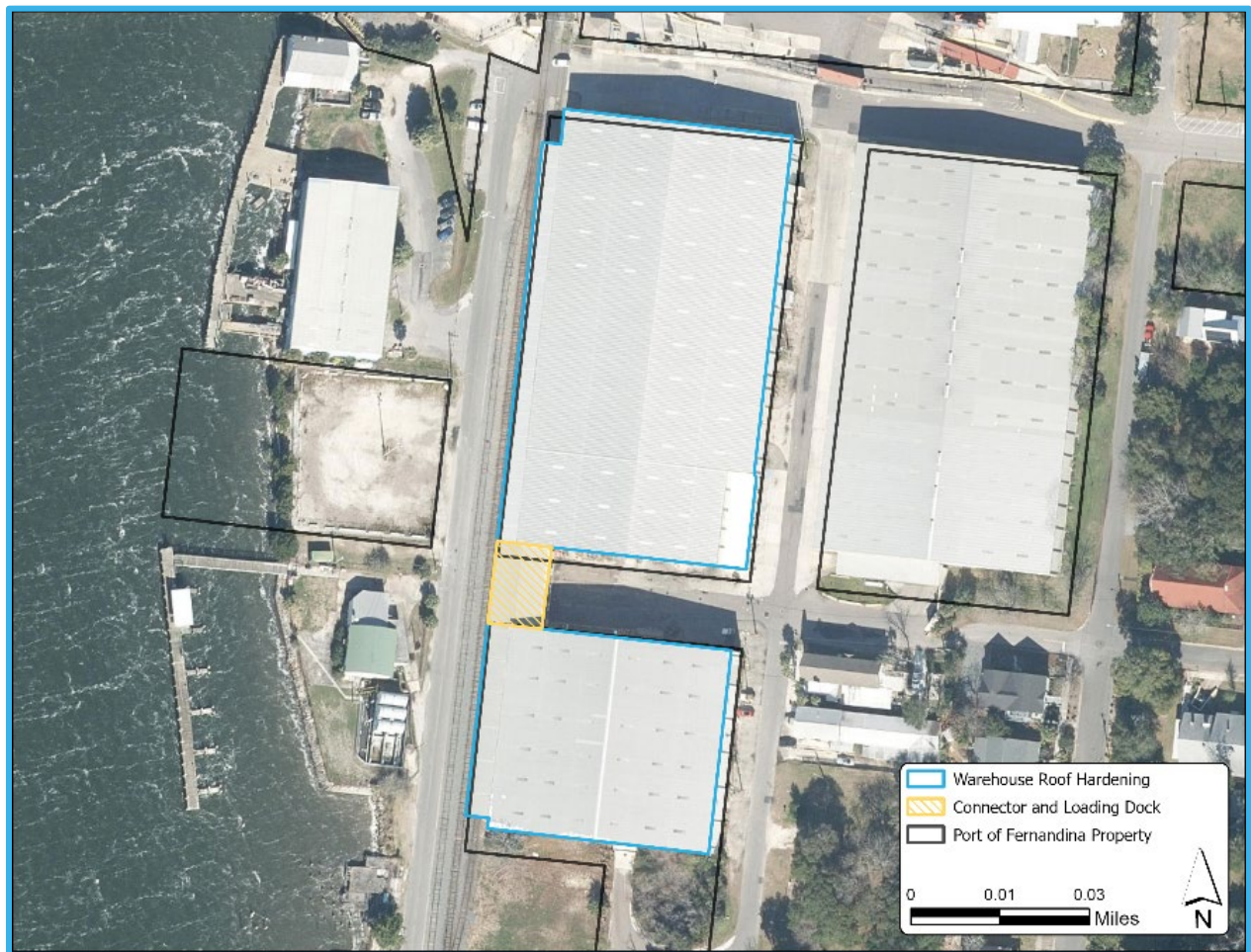
Figure 27 - Warehouse Windstorm and Hazard Mitigation Improvements
